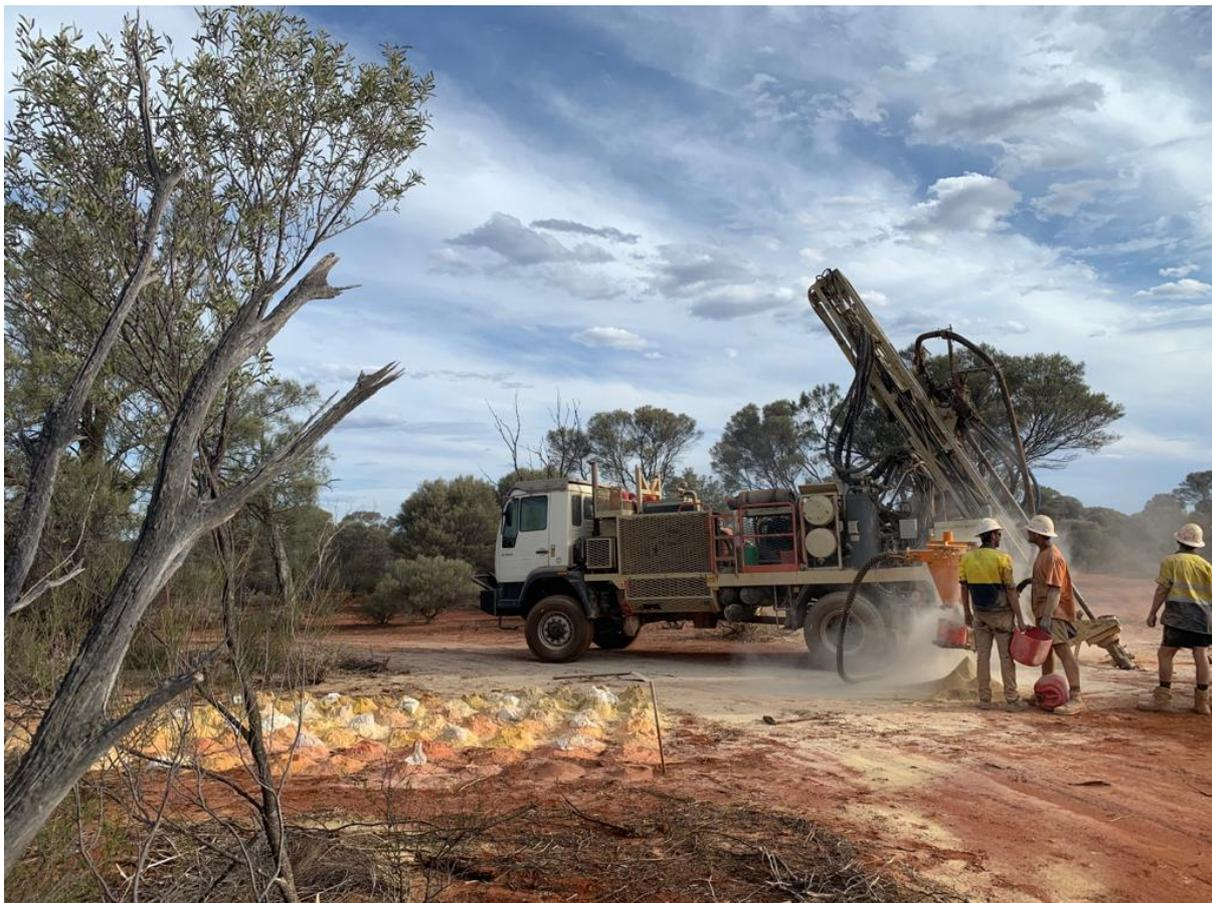
Figure 1. KTE Mining Services Aircore drill rig at Emu Lake
